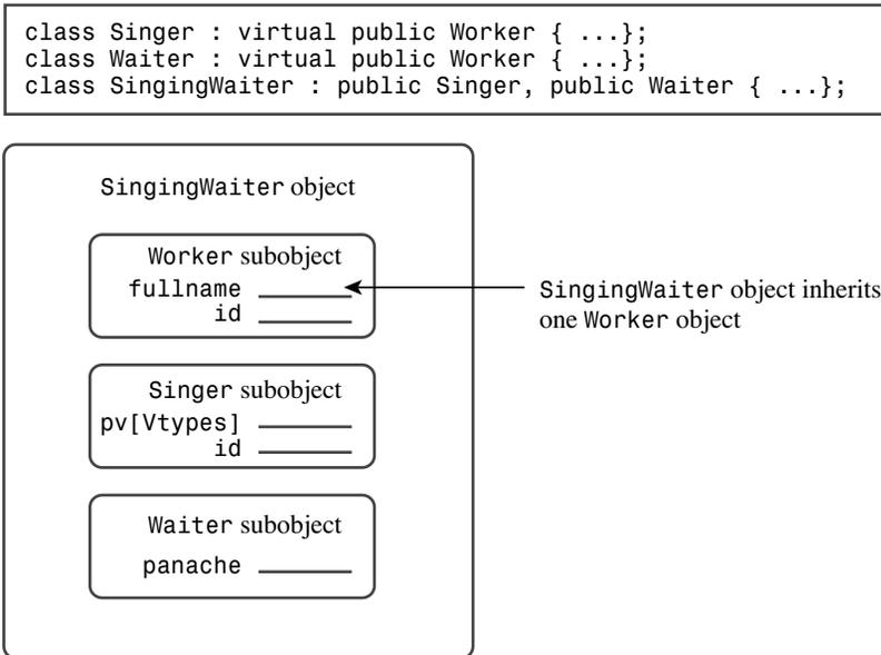
Figure 14.5 Inheritance with a virtual base class.
