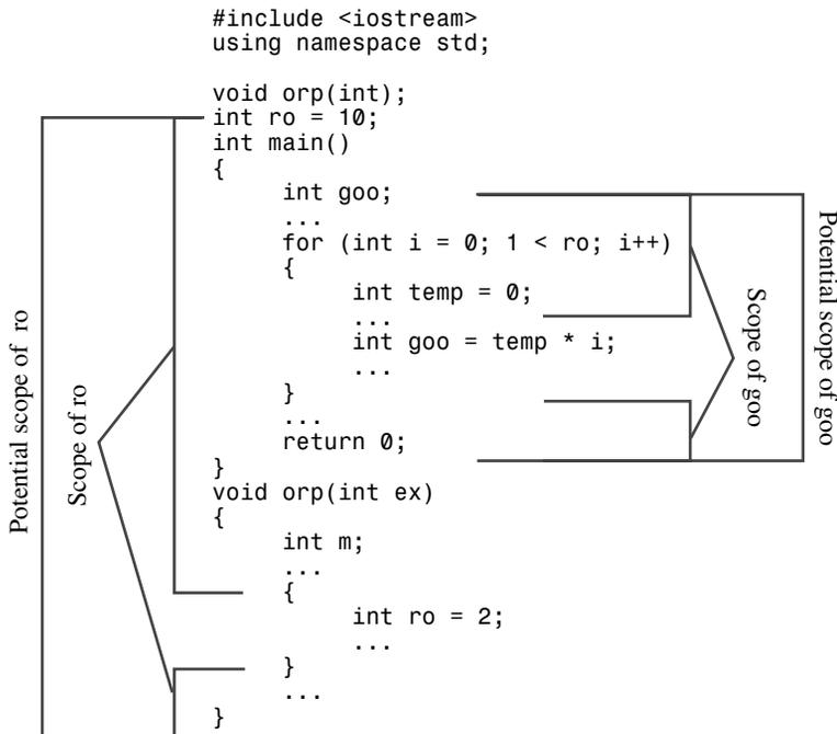
Figure 9.6 Potential scope and scope.
