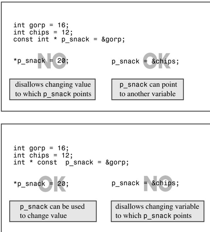
Figure 7.5 Pointers-to-const and const pointers.
