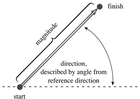
Figure 11.1 Describing a displacement with a vector.
