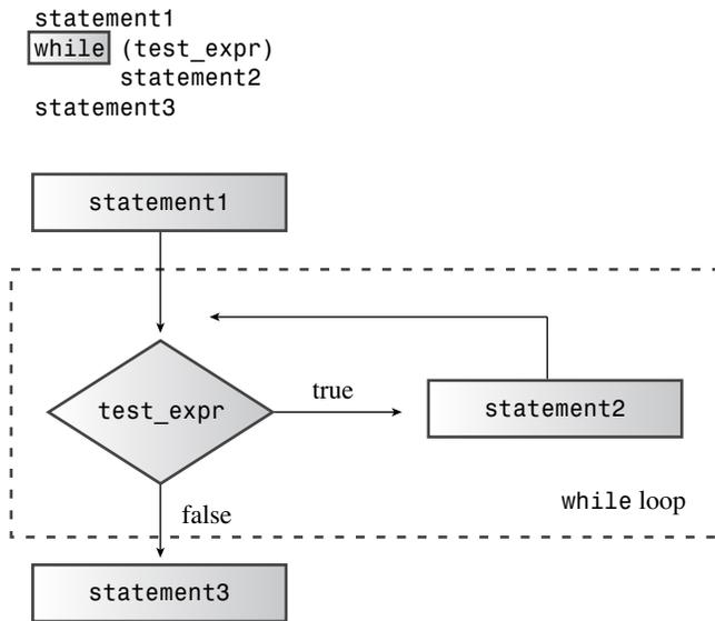
Figure 5.3 The structure of `while` loops.
