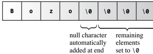
Figure 4.2 Initializing an array to a string.
