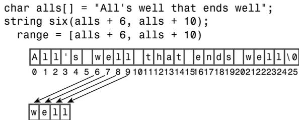
Figure 16.1 A string constructor using a range.
