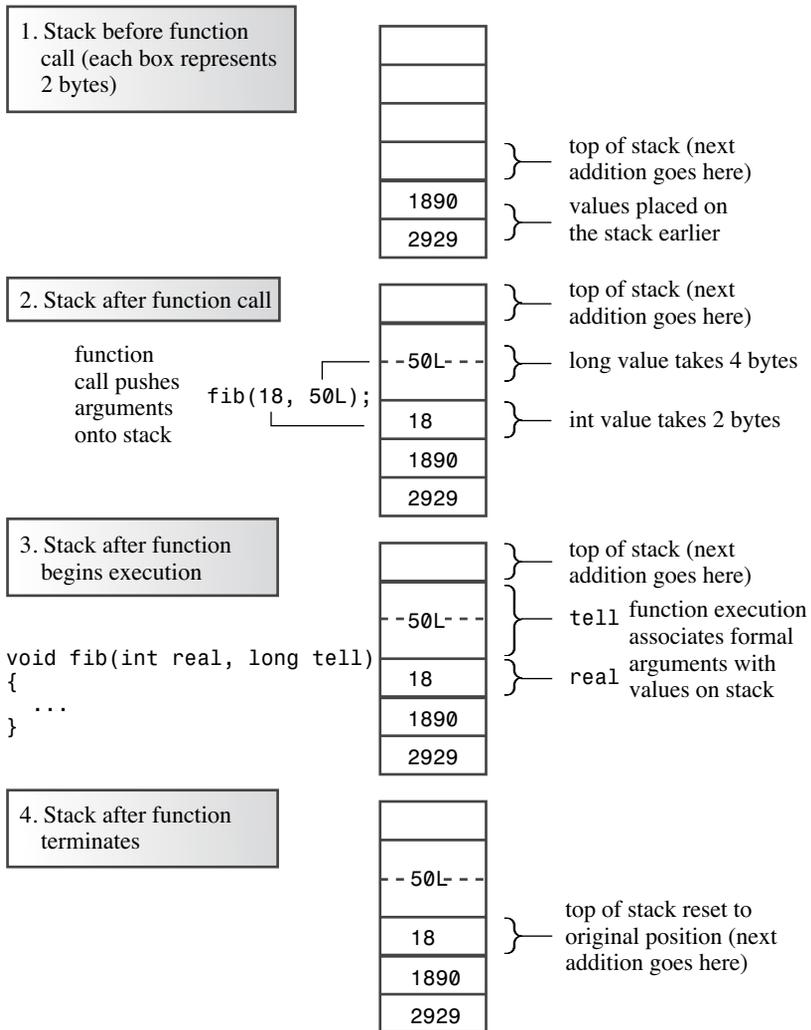
Figure 9.3 Passing arguments by using a stack.
