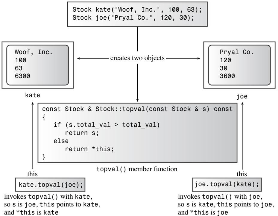
Figure 10.4 this points to the invoking object.
