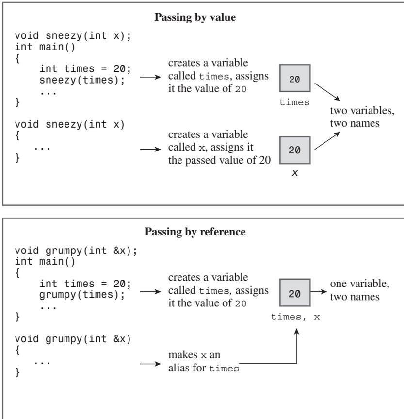
Figure 8.2 Passing by value and passing by reference.
