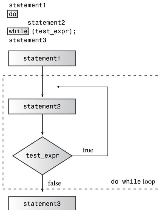
Figure 5.4 The structure of `do while` loops.
