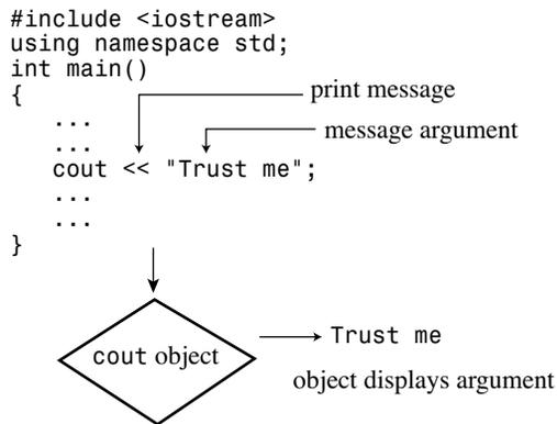
Figure 2.5 Sending a message to an object.
