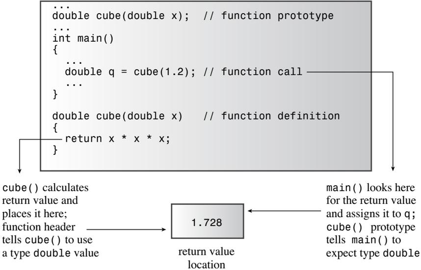
Figure 7.1 A typical return value mechanism.
