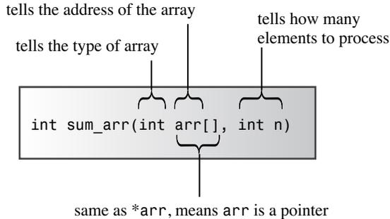
Figure 7.4 Telling a function about an array.
